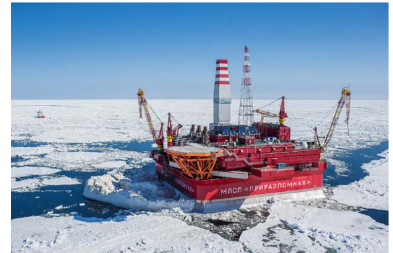
Top—Exploratory drilling in Shtokman field, one of the world's largest natural gas fields. It is located in the north-western part of the South Barents Basin. Source: http://www.gazprom.com/press/news/2012/december/article151657 . Photo © Gazprom, 2012. Bottom—The world's first offshore ice-resistant stationary oil platform (MISP) Prirazlomnaja in the Pechora Sea, operated by Gazprom Neft, 2013. Source: https://en.wikipedia.org/wiki/Prirazlomnoye_field#/media/File:МЛСП_Приразломная_зимой.jpg . CC BY-SA 4.0. Photo by Krichevsky.
