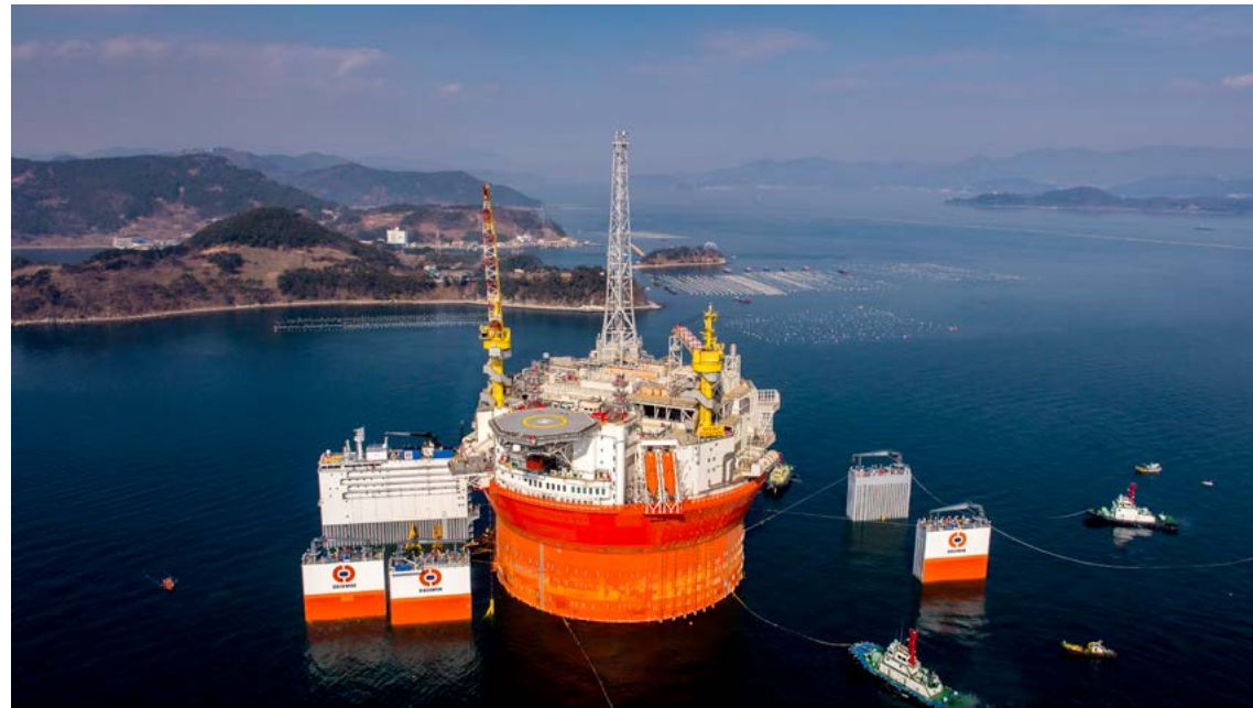
In February 2015 the Goliat platform began its voyage from South Korea to Norway aboard the Dockwise Vanguard, the world's largest heavy lift vessel. Goliat started production on 12 March 2016. Source: http://www.eninorge.com/en/News--Media/Multimedia-archive/Photos1/?dir=Goliat . Photo © Eni Norge, 2015.
