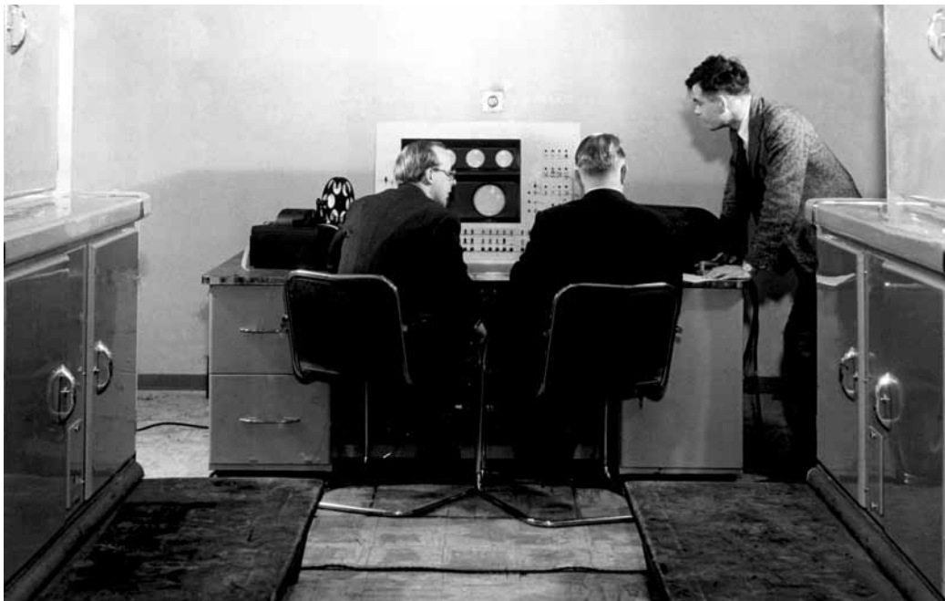
Alan Turing (standing) with Brian Pollard (left) and Keith Lonsdale (right) seated at the console of the Ferranti Mark 1 computer at the University of Manchester in 1951. The Ferranti Mark 1, with 256 40-bit words (1 kilobyte) of cathode-ray tube memory and a 16,000-word magnetic drum, was the first commercially available implementation of Turing's Universal Machine.
