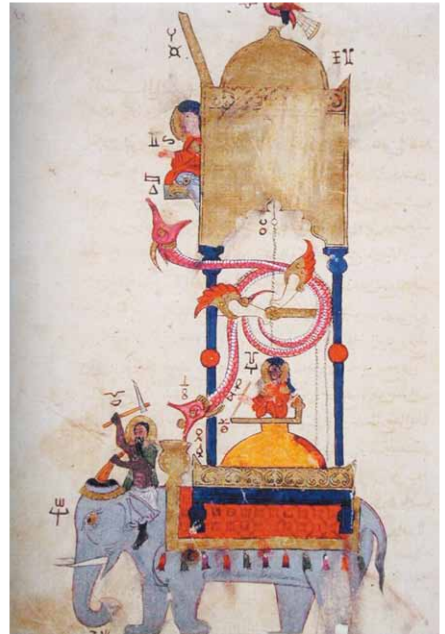
Clock: An air-powered metal bird sits chirping atop the water tank tower; below it at the front of the tank tower, flanked by two elaborate falcon heads, sits a kinetic figure moving its arms; two serpents are bound together on a central axis and turn their heads when a ball drops into the mouth of the upper one, thus shifting the serpent's weight; in the lower third of the tank tower sits a figure marking the passage of the hours on a circular metal disk; riding on the head of the elephant is the hour counter who beats time with a hammer. Drawing from a transcript of the manuscript by al-Jazari, ca. 1200.
