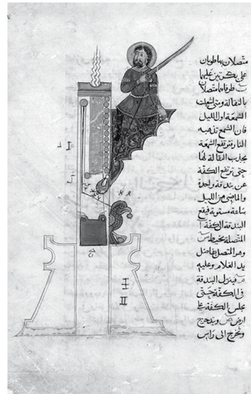
A candle clock from a copy of al-Jazari's treatise on automata, Kitab fi ma'ari-fat al-hiyal al-handasiya , Syria, 1315, dated Ramadan 715.
