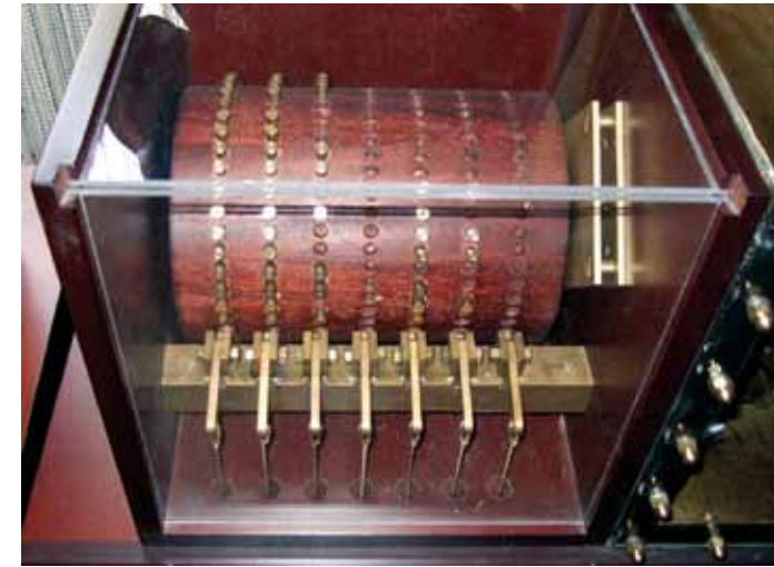
Perpetual flute player: The programmable mechanical heart of the music automaton by the Banu Musa brothers (reconstructed under the direction of Fuat Sezgin at the Frankfurt Institute of the History of Arabic-Islamic Sciences), 9th century. Photo: Siegfried Zielinski.
