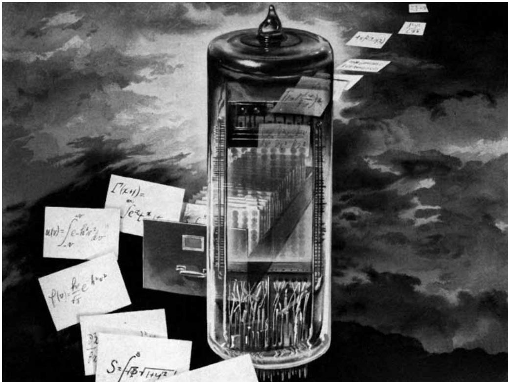
The RCA Selectron, or Selective Electrostatic Storage Tube, invented by Jan Rajchman, promised an all-digital 4096-bit electrostatic storage matrix in a single vacuum tube. The applications included numerical weather prediction, as portrayed in this advertisement in the February 1950 issue of National Geographic .
